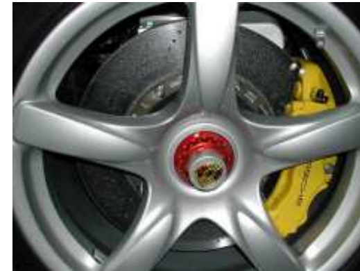
Porsche Carrera carbon-ceramic (silicon carbide) disc brake
